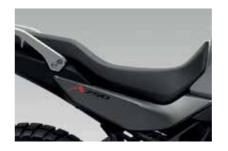
LOW SEAT \*BLACK\* 08R74-MLC-D00ZB The Low Seat, which is 20 mm lower than the standard seat, improves ground reach.
