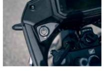
12V SOCKET 08U71-MKK-D00 Power or charge electrical equipment using this convenient 12V Socket (Provides 2A).
